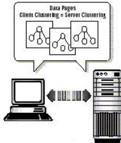
Figure 2 – Client Centric Architecture (ODBMS): Physical = Logical Clustering
